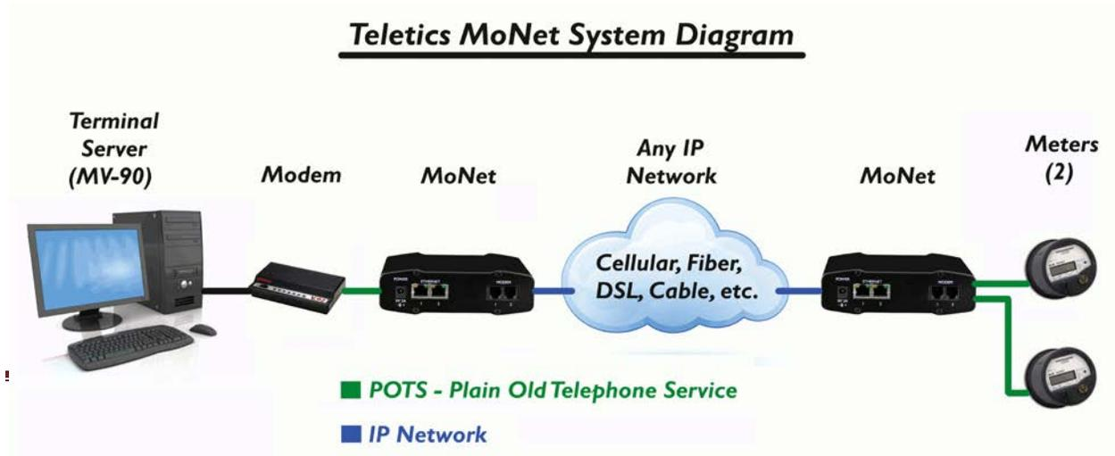
The blue cloud in the picture above refers to the internet. At the metering site, you can use any internet connection available, including cellular, DSL, cable, satellite, or any internet connection available.
