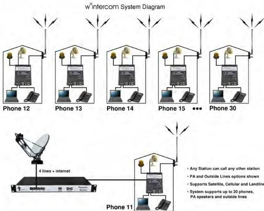
You can have up to 20 w\*intercom radios in one system. The numbers that are given to each Phone go from 11 to 30. So if the company man in trailer 13 wants to call the tool push on the drilling rig, and the drilling rig has w\*intercom 14, he simply picks up his phone and dials 14.
