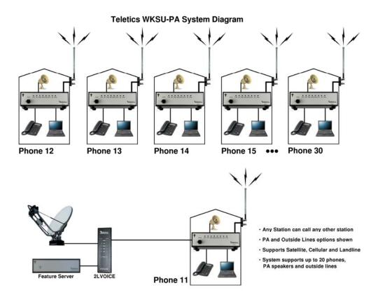
You can have up to 20 WKSU-PA radios in one system. The numbers that are given to each Phone go from 11 to 30. So if the site supervisor in trailer 13 wants to call one of the workers in the trailer with WKSU-PA 14, he simply picks up his phone and dials 14.
