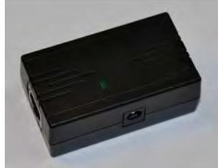
There are two RJ45 connectors on a power injector. Please ensure that the outdoor ZipLine Ethernet radio Ethernet cable gets plugged into the side that says “PoE”. This stands for “Power over Ethernet”, and is how the outdoor radio gets power. The other Ethernet connector goes to the cable to the customer's laptop, Ethernet switch or equipment. The little round barrel connector is where the power adapter gets plugged in.
