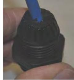
You can now slide the gland up and down the cable while you plug in the ethernet connector into the bottom of the radio:
