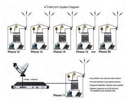
You can have up to 20 w\*intercom radios in one system. The numbers that are given to each Phone go from 11 to 30. So if the company man in trailer 13 wants to call the tool push on the drilling rig, and the drilling rig has w\*intercom 14, he simply picks up his phone and dials 14.
