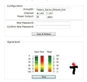
If you want to see signal strength, click on the START button underneath the colored signal strength indicator. You will then see a black signal strength indicator appear on each of the three gradient color bars, like in the example screen shot.
