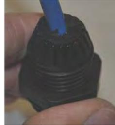
You can now slide the gland up and down the cable while you plug in the ethernet connector into the bottom of the radio:
