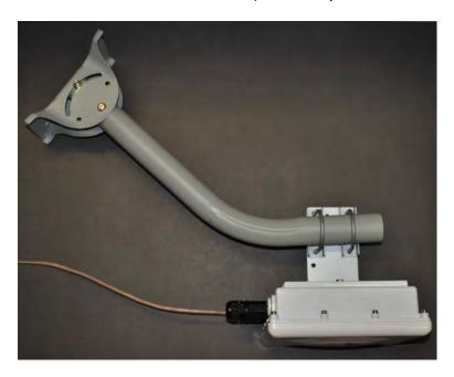
First, attach the aluminum bracket to the back of the ZipLine. Use the 4 bolts, washers, and lock washers that are already on the back of the radio:
