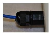
**IMPORTANT!!** – Hand tighten gland parts only - Do not use a wrench.
