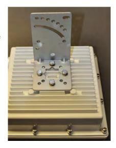
Next, put the U-Bolts in place. These are also packaged in the Accessory Kit (the white box), and are wrapped in plastic wrap, along with washers and lock washers:
