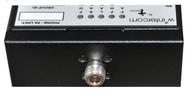
The **ANTENNA** connection is not labeled, and is by itself at the opposite end of the wintercom. It is for use with an antenna rated for 5.8GHz operation. Please contact your Teletics distributor for additional antenna and RF cable assemblies made to your requirements. This connector is a standard N Female.
