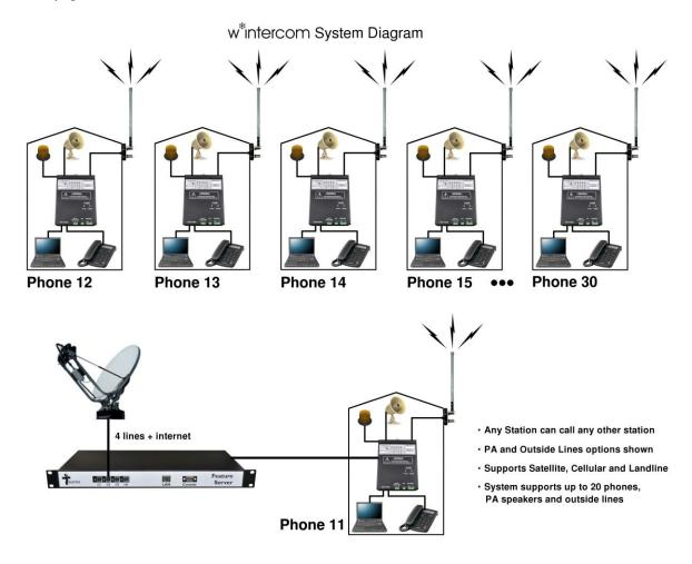
A typical installation has as many wintercom units as there are shacks or temporary structures or trailers that need to have service, and a unit in each trailer. In turn, each wintercom unit has an outdoor antenna and RF cable attached to it, plus a PA speaker (or PA amplifier), a phone and a computer.
